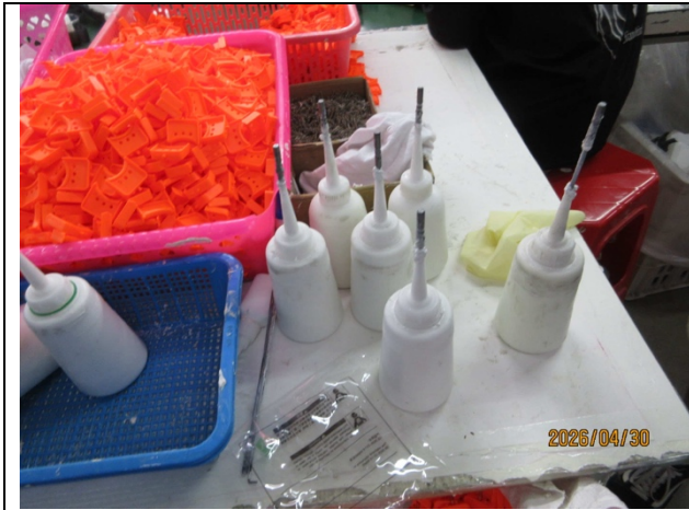
PA 7.7 No safety label for the glue used in the production area
